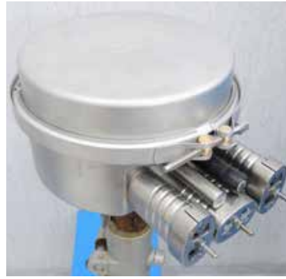
Left picture. Closure's set-up for IP6X dust test with vacuum pump connection.
