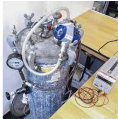
Set-up for IPX8 immersion test, water container pressurized to 2 bar.
