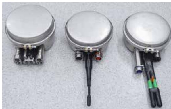
Closure's tested with all variants of bushing technology for the Telecombox T240 system.
